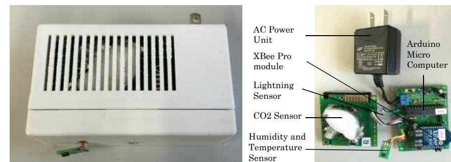
Figure 2 environment sensor device
