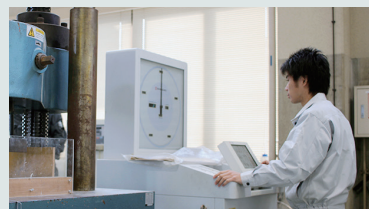
Compression test on concrete
