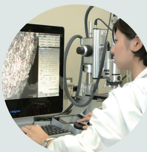
Fractographic observation with a digital microscope
