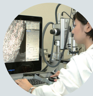
Fractographic observation with a digital microscope
