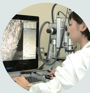
Fractographic observation with a digital microscope
