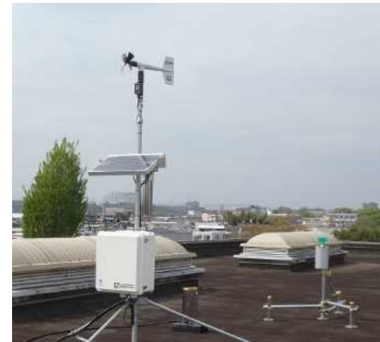
Figure 1 Automatic Weather station and rainfall sampling at Kumamoto University.
