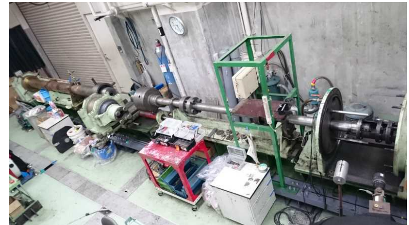
Figure 1 Two-stage light-gas gun
