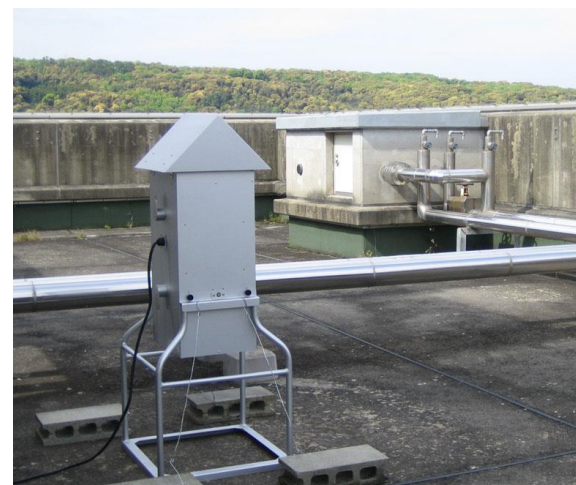
Figure 2 High-volume air sampler for chemical analysis.
