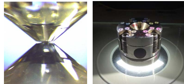
Figure 1. Diamond anvil cell. A material is squeezed and pressurized between two single crystal diamond anvils (left) in the cell (right).
