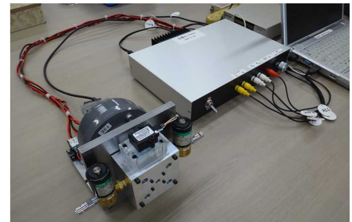
Figure 2 Acoustic leak tester.
