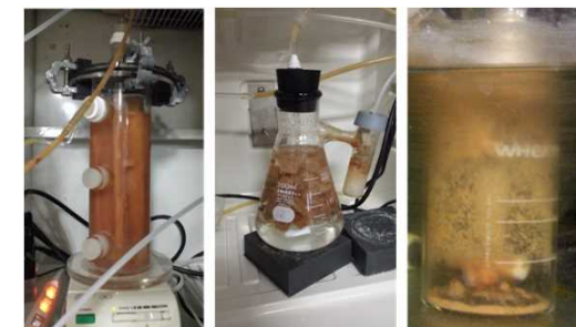
Reactor with flat nonwoven fabric Reactor with cubic nonwoven fabric Continuous stirred tank reactor (CSTR)
